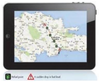
The fuel consumption monitoring report presents information about every route the vehicle has taken, from ignition and until the key switch is turned off. For each route, the report will show the fuel consumed and distance covered in Litre/Km. In addition the report will indicate points at which the vehicle was refuelled and any sudden drops in fuel level detecting a possible case of fuel theft.
